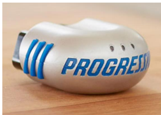
A typical dongle which plugs into a vehicle's OBD II port – in this case Progressive's Snapshot device
